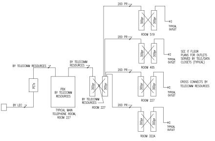
FIGURE 18.5 Typical telephone wiring diagram. (Nevling).
