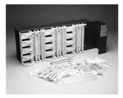
FIGURE 18.19 Lucent 110P field-terminated patch panel kit: includes wiring blocks, connecting blocks, horizontal jumper troughs, duct assemblies, hardware, label holders, and blank inserts. (*Copyright © 1999, Lucent Technologies, used by permission.*)
