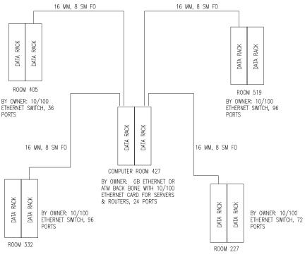
FIGURE 18.6 Typical data wiring diagram. (Nevling.)
