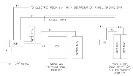
FIGURE 18.2 Typical communications grounding detail. (Nevling.)
